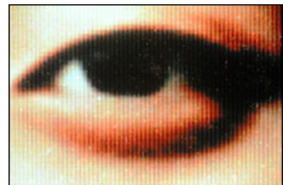
Shinko Color Stream with CMYK ribbon (RC paper, dye sublimation), 30 x magn.
