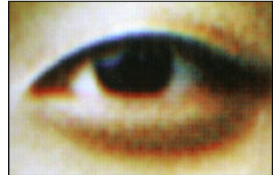
Kodak Digital Science with CMYK ribbon (RC paper, dye sublimation), 30 x magn.
